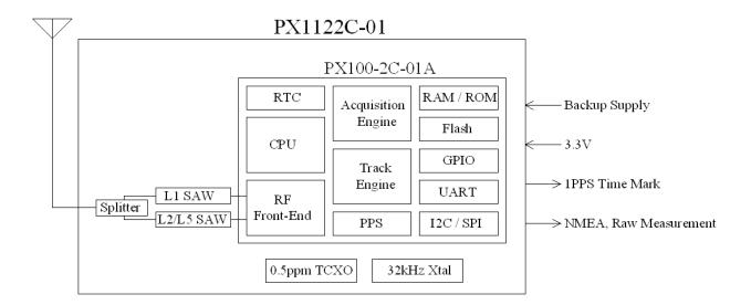
Active antenna is required to use with PX1122C. The received signal goes through a signal splitter, to individual L1 and L2/L5 SAW filters to remove out-band interference, then to the PX100 GNSS receiver chip for signal processing.
